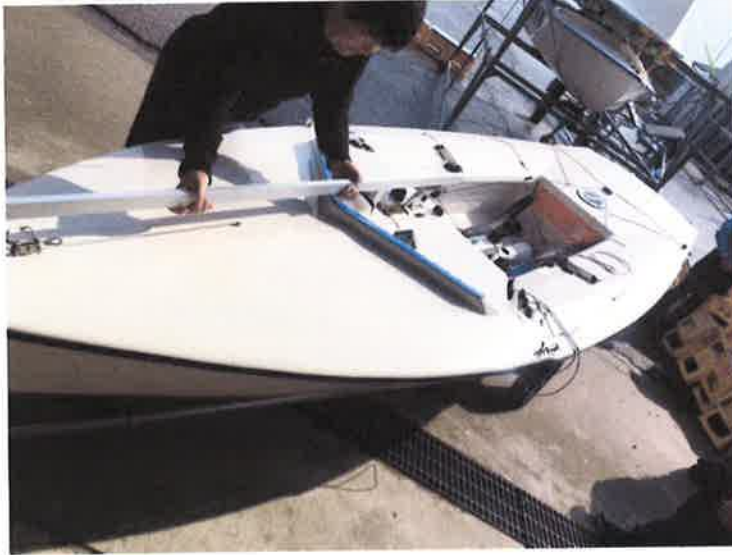
Placing jig on fore deck
