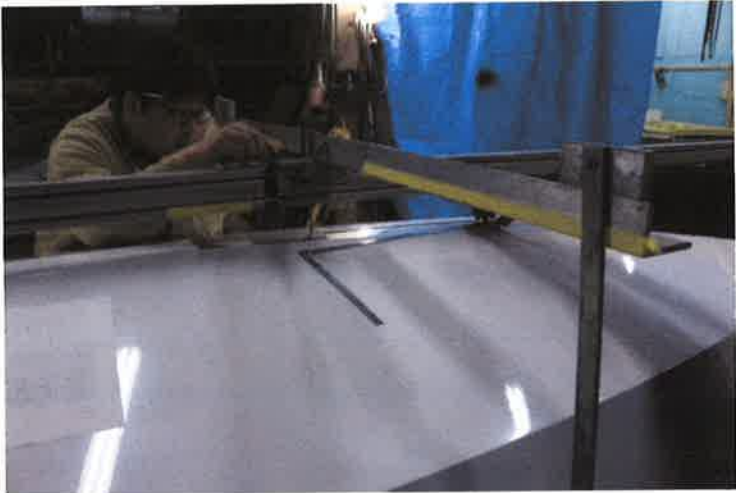
Hull measurement using jigs
