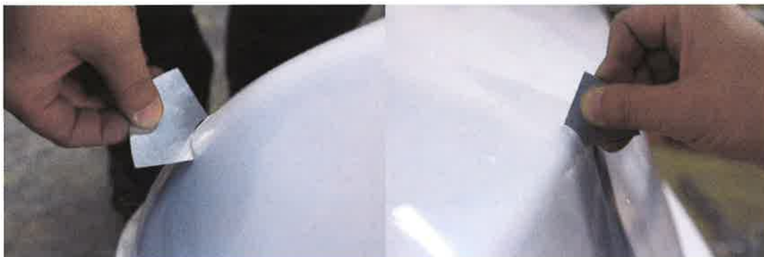
Measuring radius using a jig
